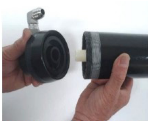
1-Line up the Ring and start threading on the Tube
