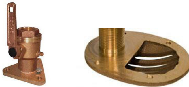
Figure 2: 3/4" Intake Seacock and Scoop, Owner Supplied
