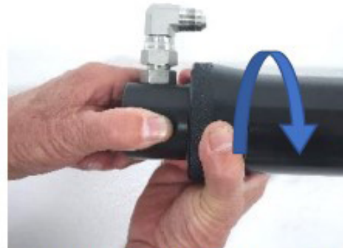
4-Finish threading the Ring on and hand tighten just snug
